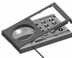
Repeat this process on the left hand or down (in case of vertical installation) hole. Lift off the cover carefully.
