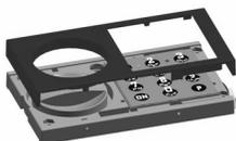
Replace the cover and press down until all four catches are engaged. Check that the lock functions correctly whilst the safe is still open.
